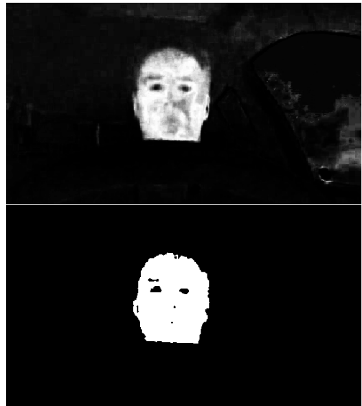
Fig. 4. Result of the color-based face segmentation as (a) probabilistic and (b) deterministic image
