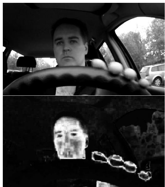
Fig. 5. More than one potential face region in the probabilistic segmented image
