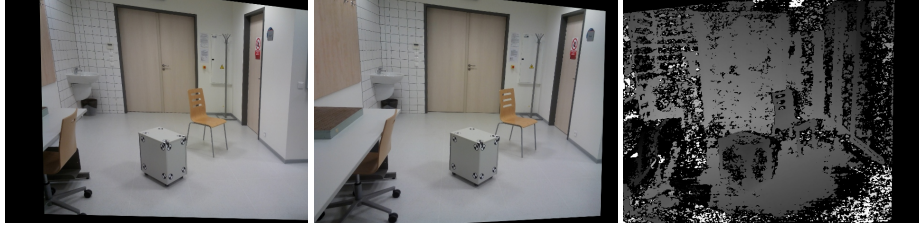
Fig. 2. Rectified images (left and middle), disparity map (right)
